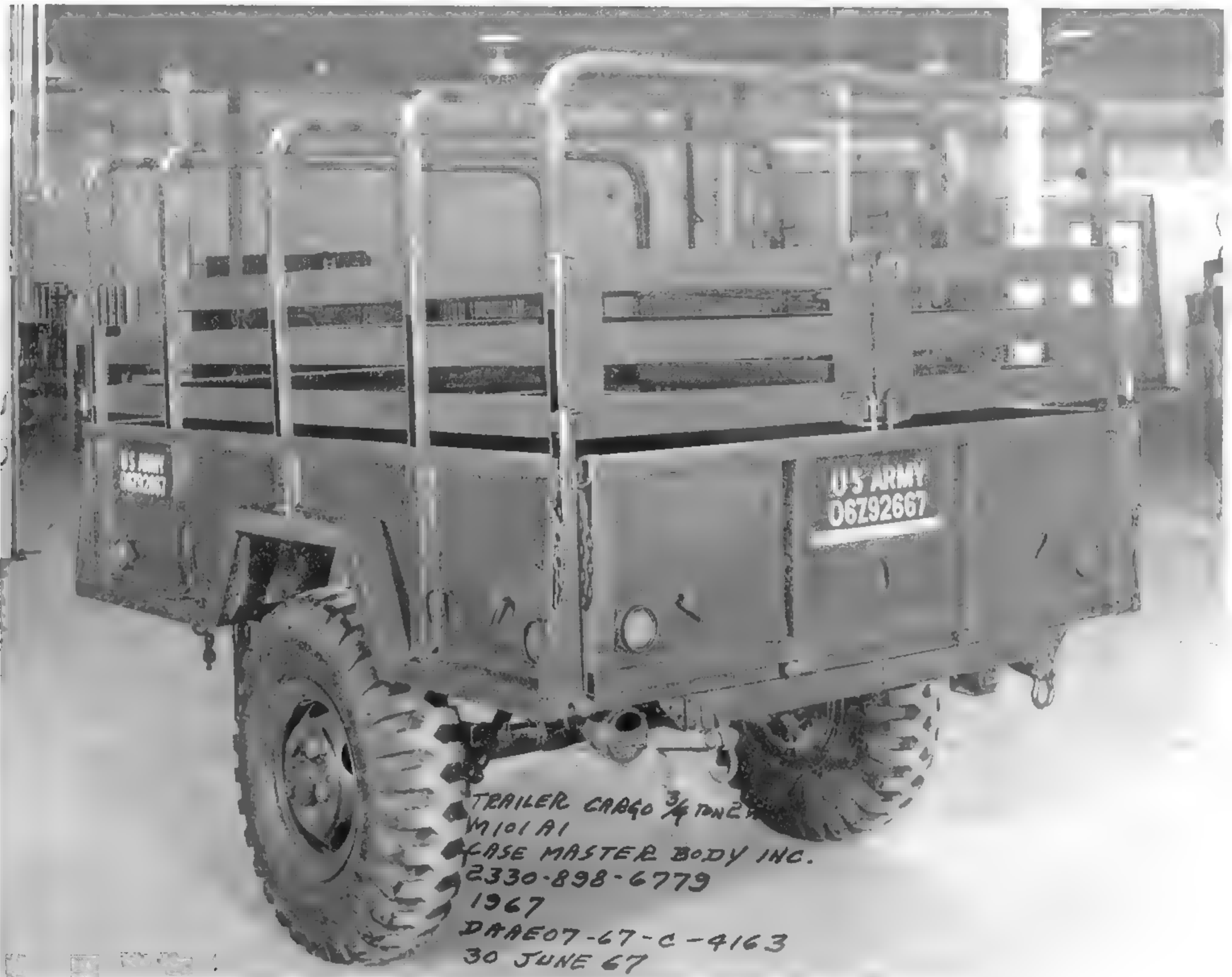
The early G-748 trailers, like this 1967 M101A1, used the same tires and wheels as the Dodge M37 truck. (U.S. Army photo)
